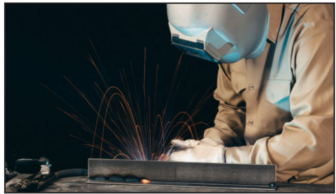
STT II Surface Tension Transfer™ reduces smoke and spatter for applications where performance is critical.
